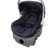
During its ongoing testing, Compass discovered a technical noncompliance issue with the crotch strap anchor located on the bottom of the seat. The metal slide used to anchor the crotch strap was installed incorrectly. In a crash, the anchor may become dislodged, allowing the child to move and increase the risk of serious injury.
